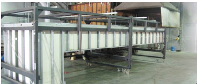
FM 4924 Fire Pipe test
